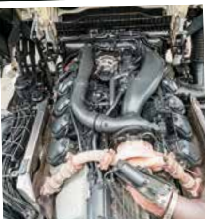
The Scania V8 cylinder firing sequence is 1-5-4-2-6-3-7-8, giving it a distinctive growl.
