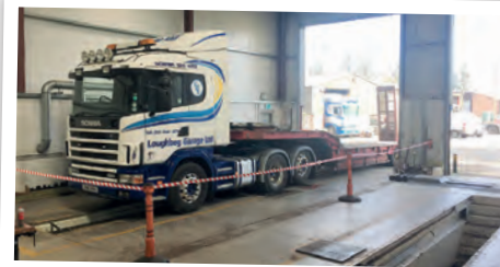
Truck undergoing dynamometer testing.
