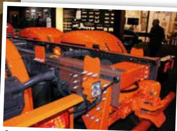
Everything that's orange on this 8x4 chassis can be cut, adjusted, added or moved to suit bodybuilder and operator requirements.
