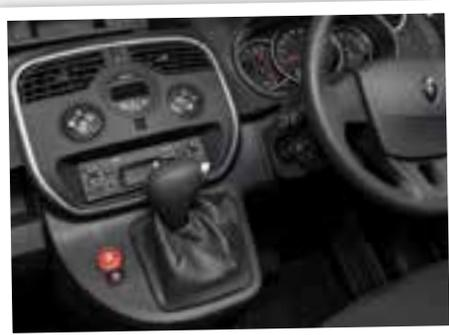
Renault's Efficient Dual Clutch (EDC) automatic transmission has been introduced to the Kangoo range for the first time.
