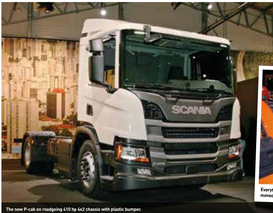
The new P-cab on roadgoing 410 hp 4x2 chassis with plastic bumper.
