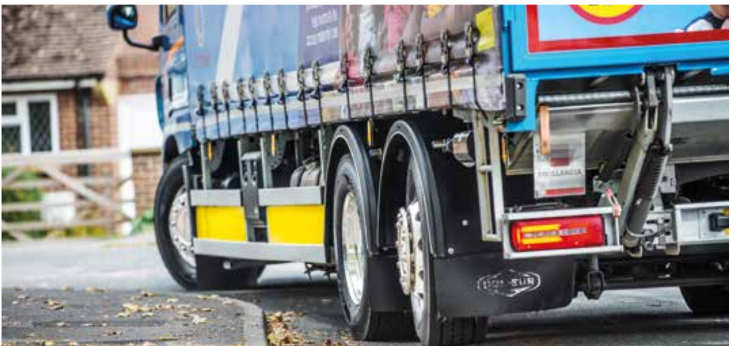
The turning circle of the 6x2 FAN rear-steer is 20.92metres, which is 1.46metres smaller than the 6x2 FAR fixed axle rigid.
