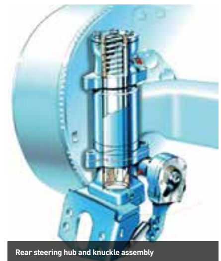
Corrugated washers at rest (steering straight ahead). Self steer
