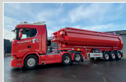
New Fruehauf Agri Trailer for Robinson Concrete, 32 cube trailer on SAF Disc axles with Auto Cover supplied by Granco.
